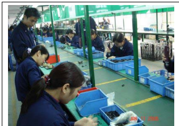
RC Car assembly line; note the conveyor belt in front of the workers
