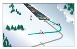
of wing flaps used. When there is a strong wind on final approach or the flaps will be used to produce a steep angle of descent, the base leg must be positioned closer to the approach end of the runway than would be required with a light wind or no flaps.
