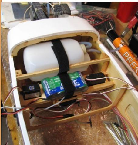
I have pulled the existing air lines out to clean up the tangle and run them straighter from/to their connections so things are in an intermediate state there just now. I found a new, 16-ounce fuel tank that has been installed and plumbed to the fill and feed lines as well as the vents. I expect to get an engine test in the near future. I have added a new battery mount to support a 3600 mAh pack and installed a heavy-duty switch assembly.
