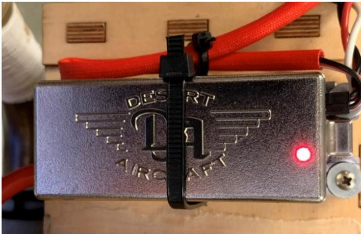
When the motor is running the light looks mostly green with a red crescent at the top. Because of vibration and proximity to the running propeller, the following picture is terrible, but it gives an idea of what to look for.
