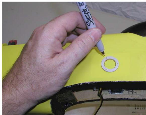
3. Use the Nut Ring as a template for marking the hole location, and trace out the inner diameter and the three screw locations, as shown to the right. Cut out the circle and the three holes and test fit the base.
