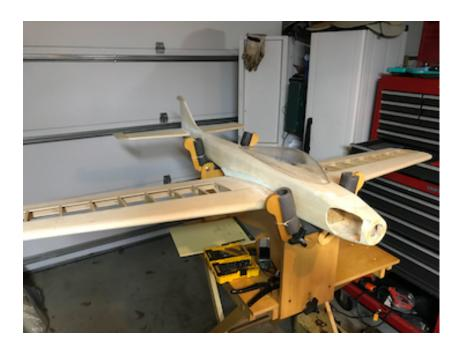
This is the "before" picture with the cowl set up for the nitro motor. For the electric version a new cowl will be needed. I had moved the firewall back in order to make room for a pumped version of the 61 SF, so the firewall also needs to go back to its original location in order to make more room for the battery.
