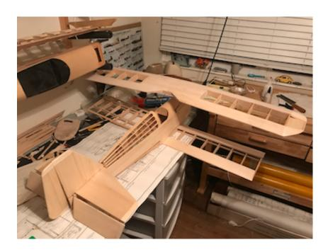
The next project is a Joe Bridi Dirty Birdy pattern plane built from a Bluejay kit. I had it set up for an OS 61 SF nitro motor, but have since decided to switch it to electric. That necessitated some surgery.
