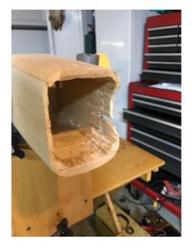
Out came the hacksaw off came the old cowl... Next I had to remove the old firewall by drilling holes all the way around it. Tedious and somewhat messy, but I got it done. Finally, a new firewall has been cut and mounted temporarily.
