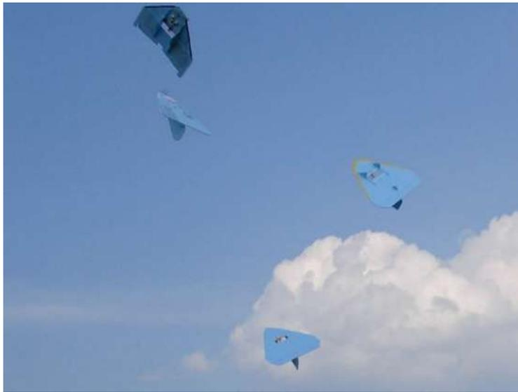
One thing to ALWAYS remember, the tail fin is on the BOTTOM when the plane is flying normally, it looks like it's flying upside down. When you launch the plane, make sure you don't have the fin up and pull back on the elevator thinking it's going to go UP! It won't! I know this from experience.
