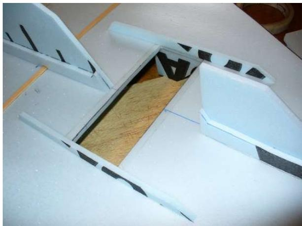
Glue the tail fin and nose fin onto the body of the plane using the hot-melt glue gun. Insure the fins are aligned dead center of the body and not angled in any way. At this time, you can also add the other reinforcement strips. These are just strips of foam cut and glued along the bottom of the fins and along the sides of the propeller cut out.
