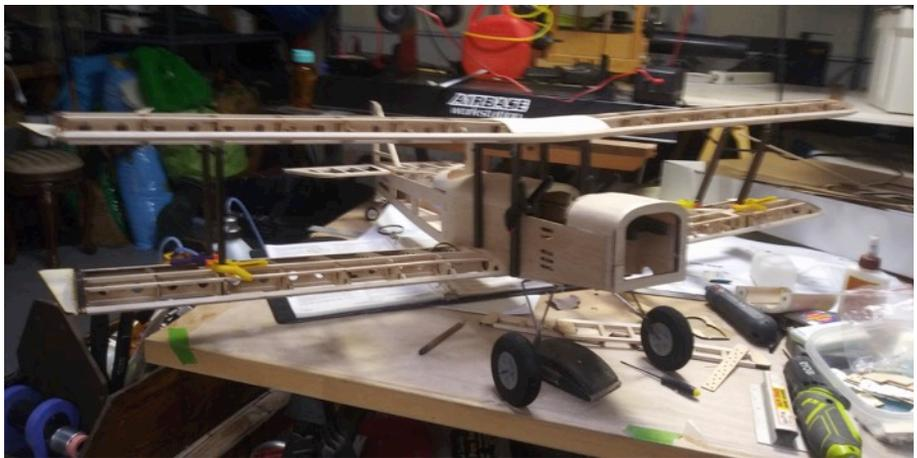
Specifications: Wingspan: 46.5 in. • Wing Area: 725 sq in. Airframe Length: 34 in. • Weight: 3.5 - 4 lbs. (ready to fly)
