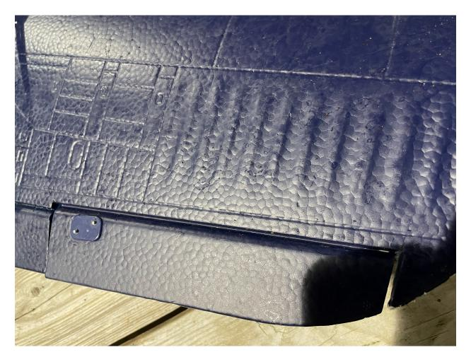
Many new foam planes do not have ANY HINGES. They use a narrowed down section of the main foam, perhaps 1/8" thick, at the control surface joint.
