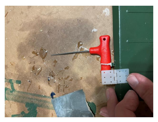
Alternate strip type hinge with even more holding power. Note any time you install new Robart type hinges or this strip type, I recommend 30 minute epoxy glue and a liberal coating of Vaseline at the actual joint to prevent the epoxy or any glue from locking the hinge joint.
