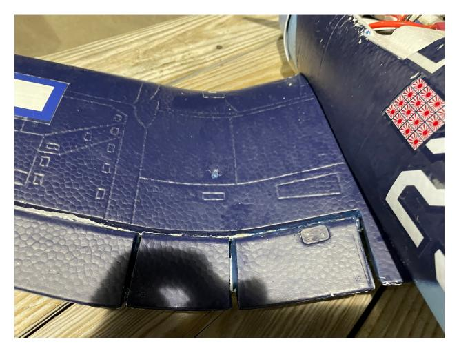
As the joint begins to fail, you will see more and more different color at the control surface to wing joint. Soon it will begin to tear. If not inspected with will fail.
