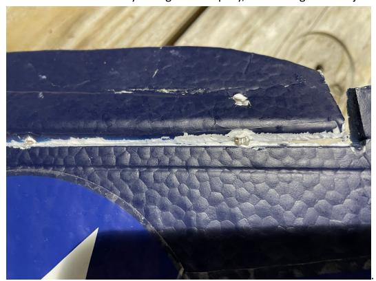
You can see the joint previously failed and ripped apart. This is a permanent fix.
