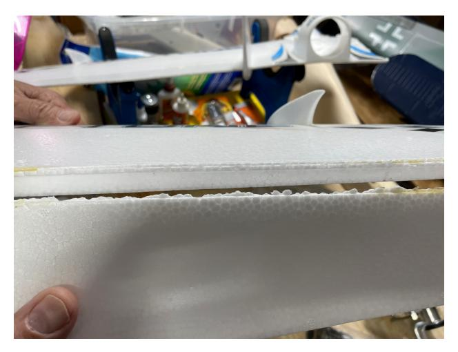
This is an example of a failed aileron joint on a glider..............I PULLED FROM THE TRASH can. It is not a matter of "IF", but "WHEN" this will happen. So carefully inspect or pull on these joints regularly.
