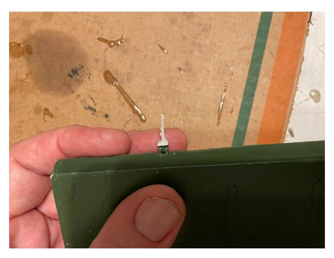
This tiny hinge is only one of three holding a 12x3" aileron to an 80" ARF.
